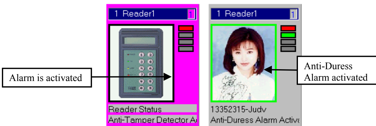
Figure 2.11 · Reader Error Status
